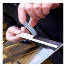
First take the steel tapes from the back of the edging as it is easier to cut with scissors. It needs to be cut square, not mitred.
